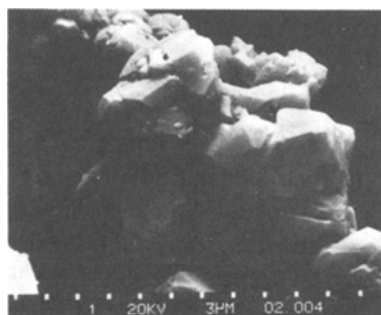
Fig. 6 Scanning electron micrographs of crystalline [\text{Co}(\text{NH}_3)_6]\text{Cl}_3 powder (magnification 3000\times )
